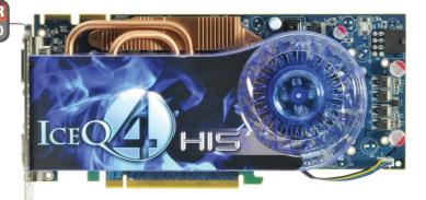
from 675MHz to 685MHz, while the cooling system works beautifully using a mix of heat pipes, enhanced and isolated heatsinks and a dualslot design that efficiently channels hot air out of the case.
